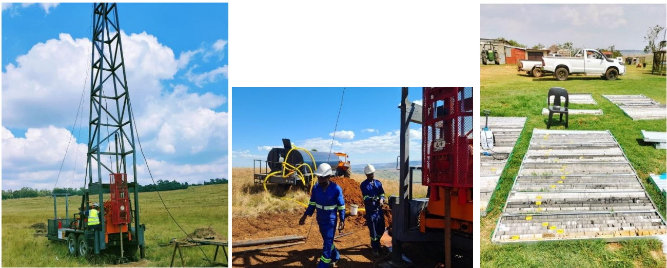
Figure 4: Typical example of exploration drilling (diamond core) and sampling (core logging).
