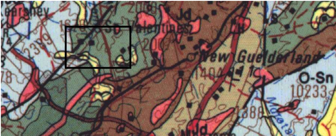
Figure 2: Approximate area (boxed) of the Shakaspring Subsidised Housing project. Extract from the 125 000 Geological Map: Durban 2930. According to this map, this project will intersect Dwyka Group (C-Pd:Greenish), possibly the Natal Group (Light Blue) and Karoo Dolerite (Jd: red).
