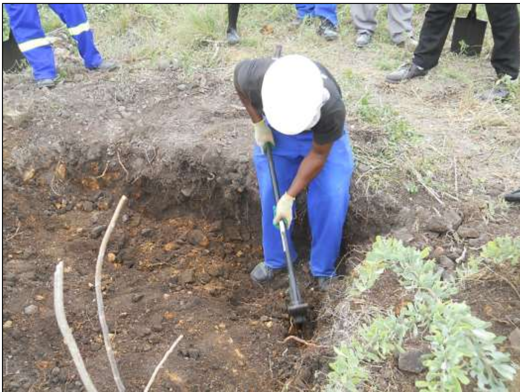
Figure 3. The test trench is expanded. Note yellow decomposed granite as bedrock.
