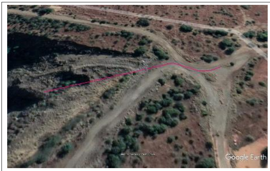
Figure 5- The K3 Tailings Bypass is a short pipeline added to the K3 Tailings to the Booster Pump Station pipeline corridor. It crosses an intersection of several dirt roads and then descends into Void 5 (above).
