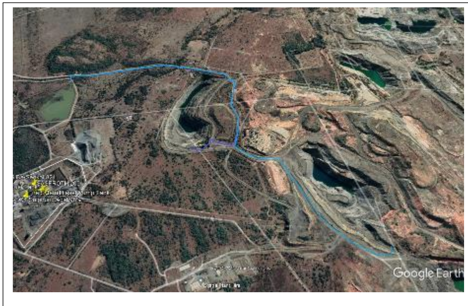
Figure 11- Both these stretches of pipeline (dark blue) follow the shoulder of a haul road at the top whilst the lower part crosses intensely disturbed mining areas (above).
