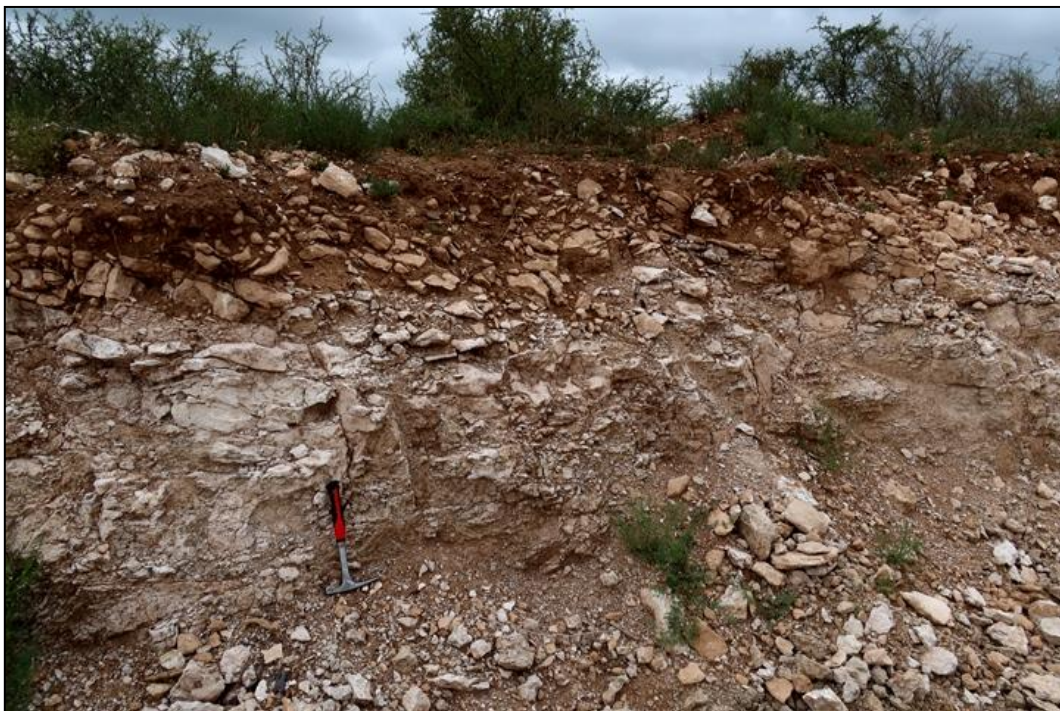
Figure 16: Thick sandy calcrete hardpan exposed on the margins of a shallow quarry in the central sector of the Remainder of Farm 632 and capped by dark brown soils with abundant calcrete rubble (hammer = 30 cm).
