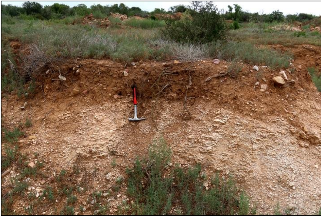
Figure 17: Well-developed calcrete hardpan beneath gravelly brown soils exposed in a shallow quarry area in the south-eastern sector of the project area (hammer = 30 cm).
