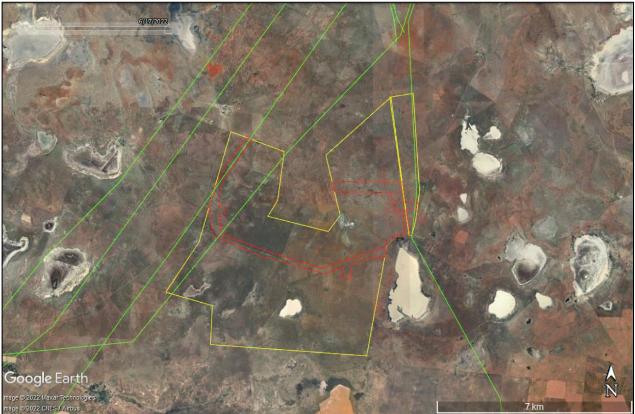
Figure 5: Existing HV lines (green) in the vicinity of the broader study area (yellow) and grid connection corridor (red).
