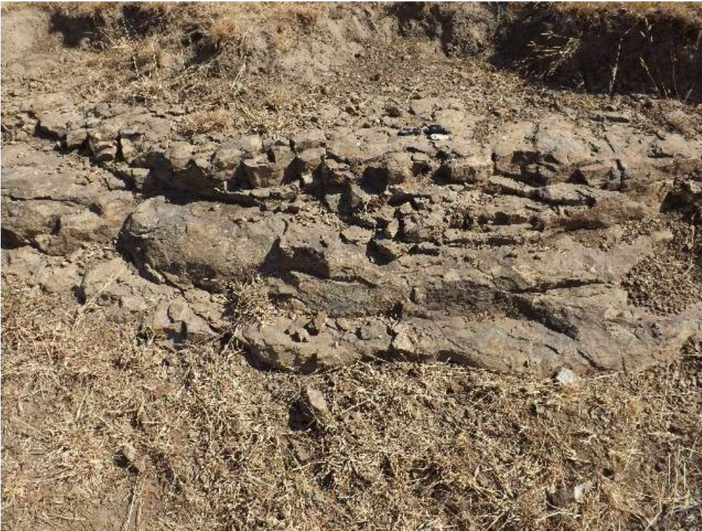
Figure 3: An example of the Estcourt Formation as it could occur in the proposed development area. However this lithology is expected to be deeply weathered on this site, but there could be fresh rock at depth (>2m).
