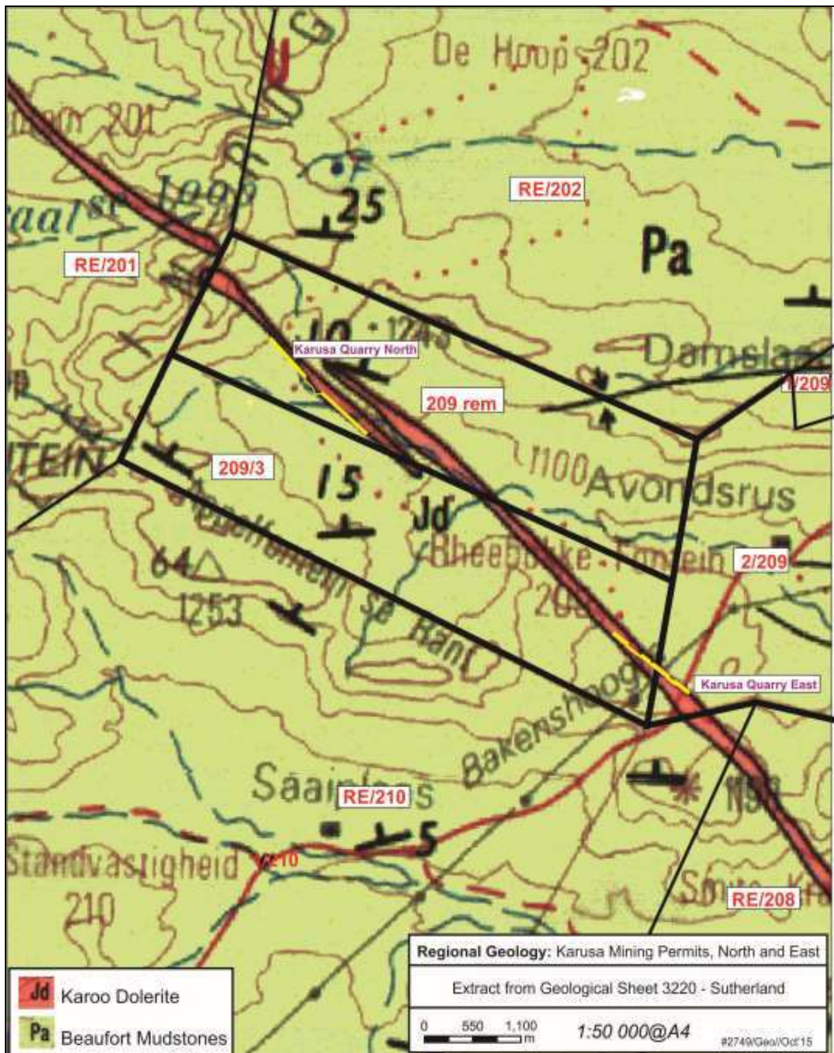
Fig. 8. Geological setting of the Karusa North and Karusa East borrow pits (yellow lines) on Farm Rheebokke Fontein 209 based on the 1: 250 000 geology sheet 3220 Sutherland (Council for Geoscience, Pretoria) (Image abstracted from the Scoping Report by Site Plan Consulting (Nov., 2015).
