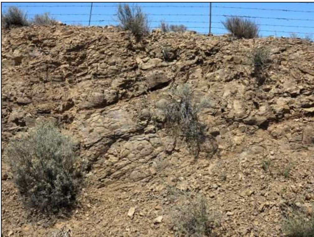
Fig. 2. Deeply-weathered, friable dolerite exposed in the walls of an existing trench-like borrow pit on Farm Karreebosch 200 (R354 borrow pit site).
