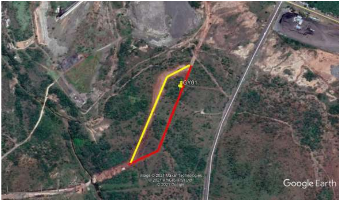
Figure 6: Aerial view of the realignment of New TSF pipeline in yellow, the old proposed line in red and identified graves marked GY01.
