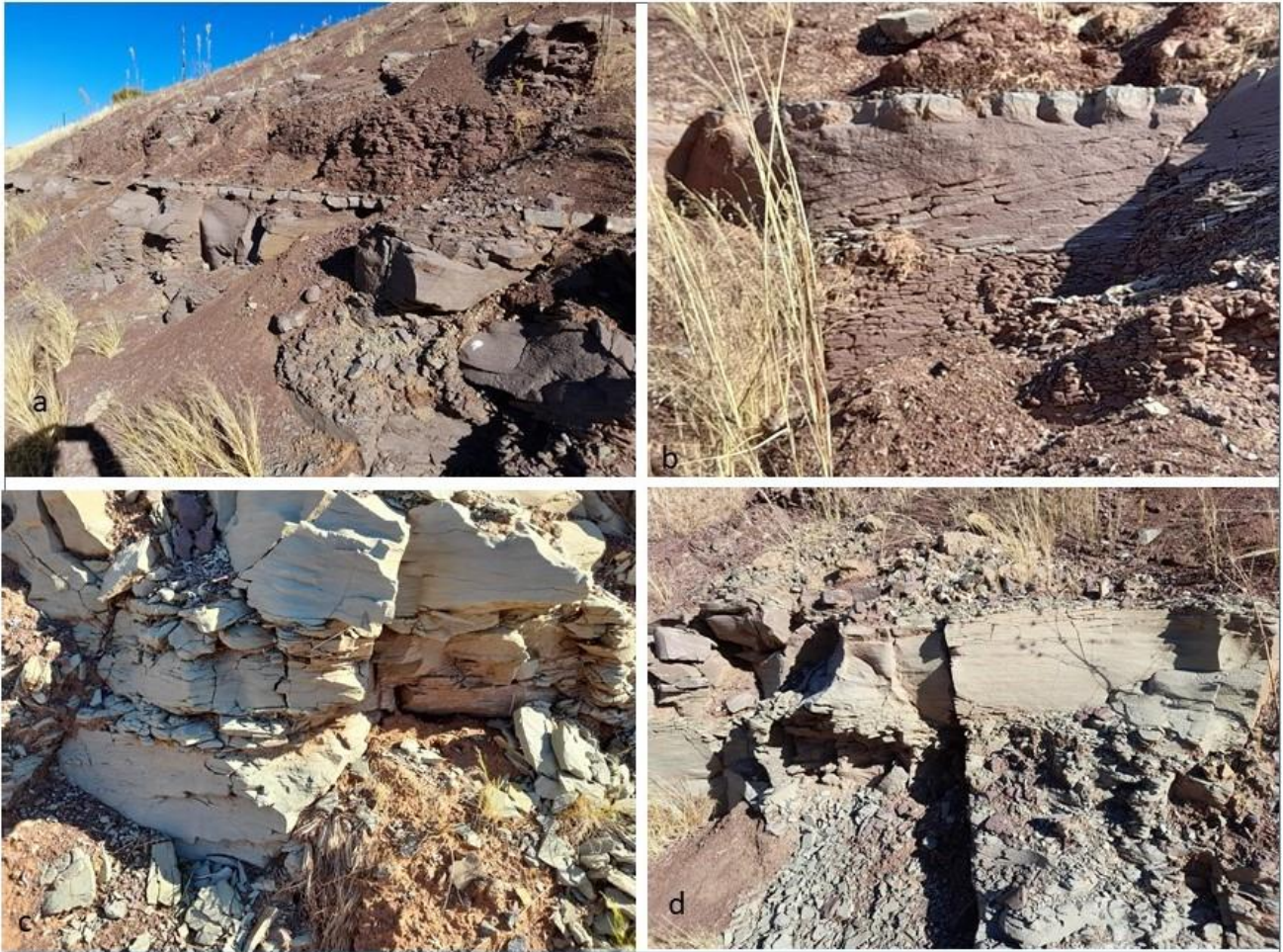
Figure 10: Road cutting on the N6 (Stop 18) just to provide an indication of the type of rocks being looked for as they are mudstones of the Tarkastad Subgroup but did not have any fossils; a, b – massive mudstones with thin cappings of sandstone overbank deposits; c, d – finely laminated mudstones fracture and weather rapidly when exposed to the air.
