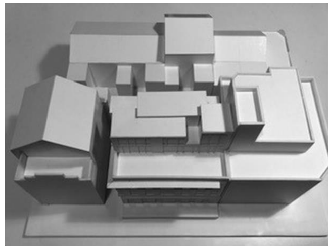
KFA DEVELOPMENT PROPOSAL FAÇADE TO BUILDING LINE, STAGGERED SETBACK TO THE REAR, A CORNICE WITH OPEN SIDE SPACE WHICH ALL WHITTLE THE FLOOR AREA DOWN BY A THIRD
