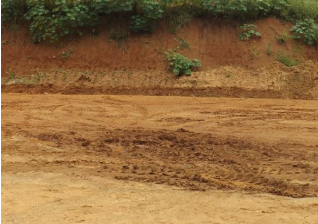
Figure 3: Earth cut showing the characteristic appearance of the Umkwelane Formation (Berea Red Sand).
