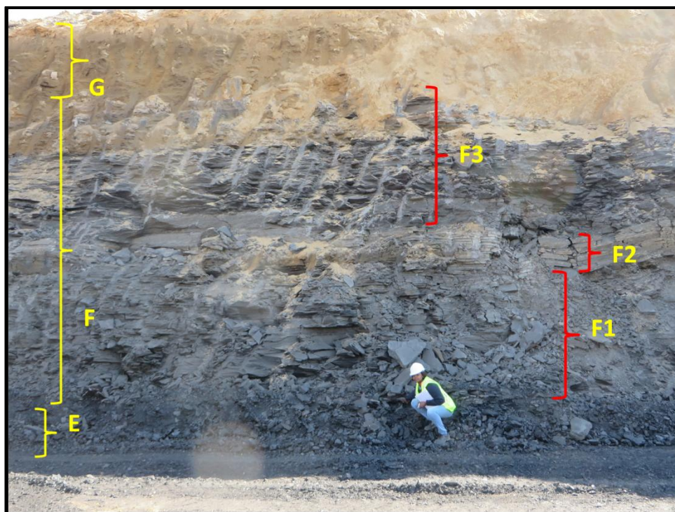
Figure 7: The lithological sequence present in cut 7 (see Table 2 for terminology). Ms E. Nethavhani of Vaalbult Mining Company (Pty) Ltd has her right hand located on the contact of unit E and unit F. Unit F is subdivided into three distinct lithological subunits. At the base is ca. 2 m of laminated to massive, grey mudstone (F1), which is overlain by ca. 1 m of thinly light grey mudstone (F2), and an upper-most ca. 2 m of black, carbonaceous mudstone (F3).
