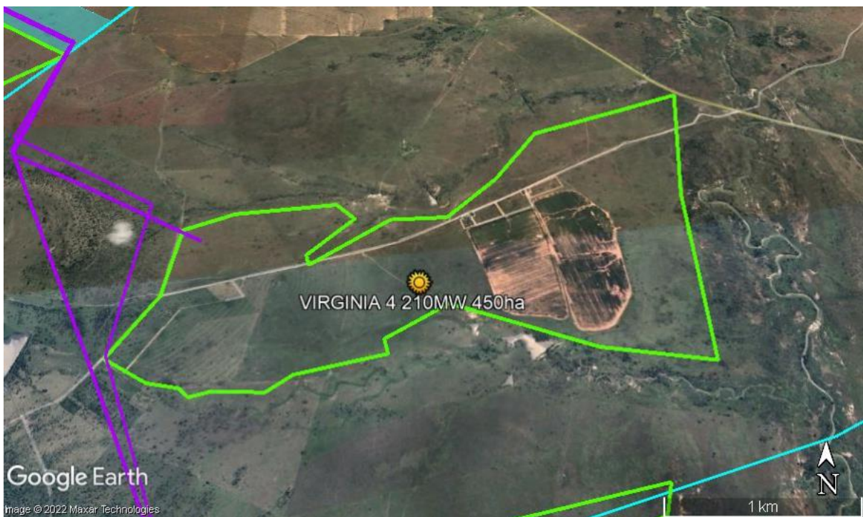
Figure 2: Google Earth map for the proposed Virginia 4 Solar Park (green outline) and the grid connection (purple lines).
