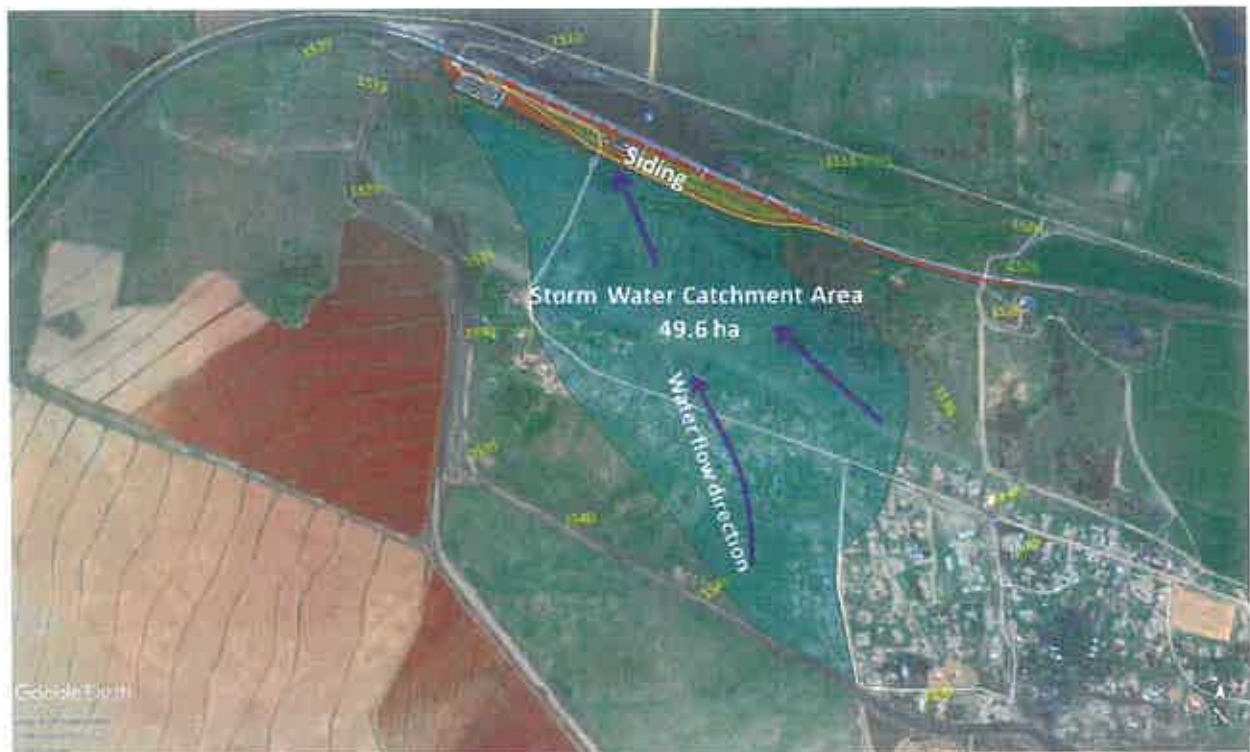
Figure 14: Storm water catchment area
