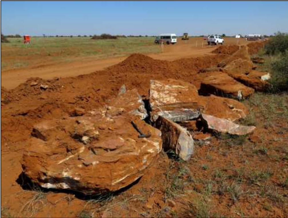
Figure 15: Large blocks of Boomplaas carbonate bedrock recently excavated from V-drain trenches showing persistent patina of soil and extensive scratching (Loc. 338) (Hammer = 30 cm).
