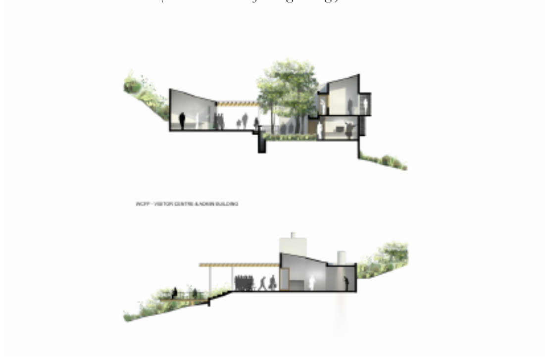
FIGURE 3: Cross Section of the proposed administration and restaurant sections linked by an internal “street”. Noero Architects 2013 (See Annexure 8 for larger image).
