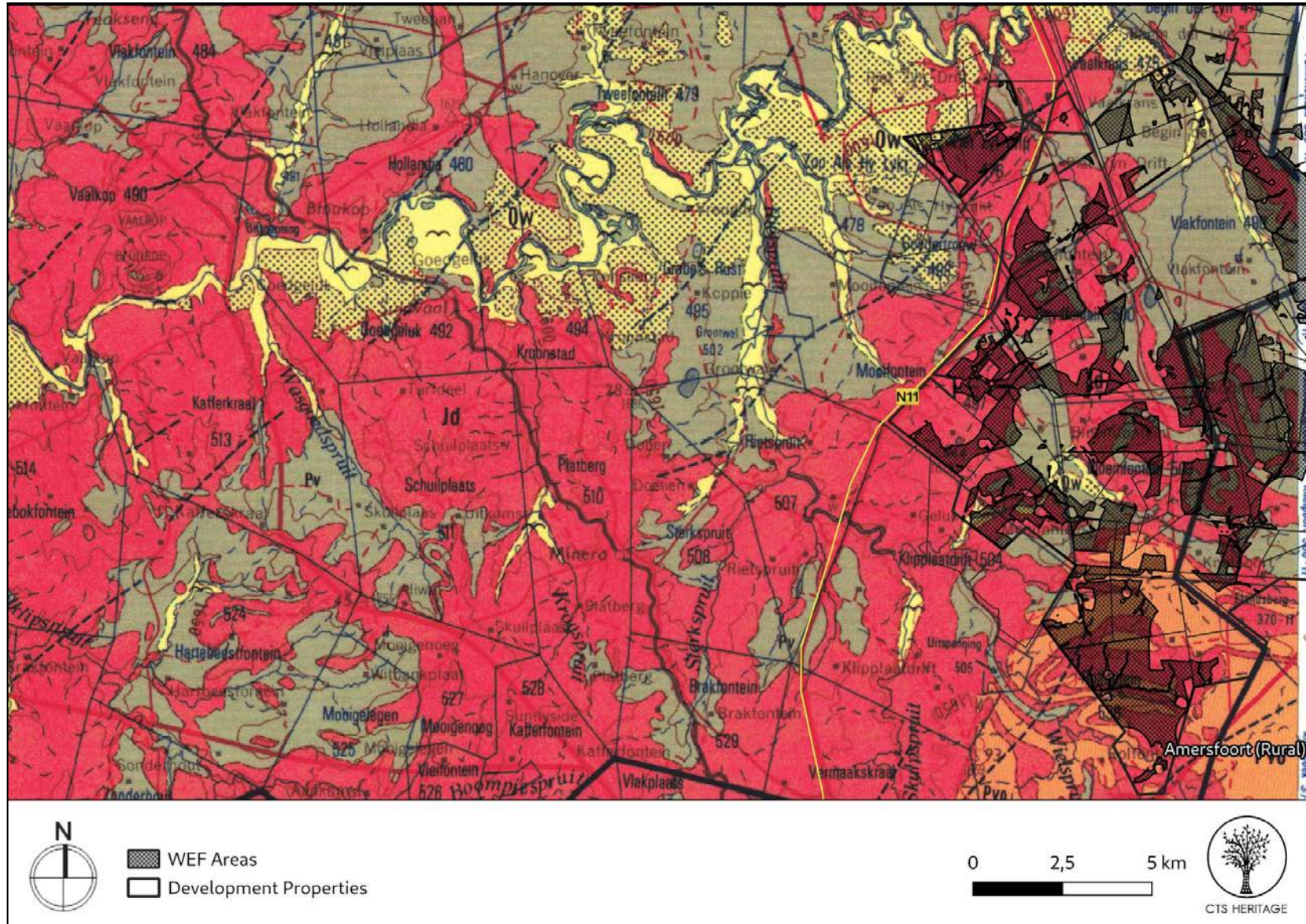
Figure 4b. Geology Map. Extract from the CGS 2628 East Rand Map indicating that the development area for the REF development is underlain by sediments of Pv: Vryheid Formation of the Ecca Group and Jd: Jurassic Dolerite as well as the Pvo: Volkruis Formation and Quaternary Sands
