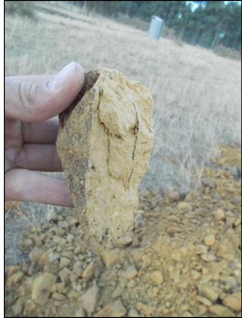
Note: Soft rock shale fragment.
