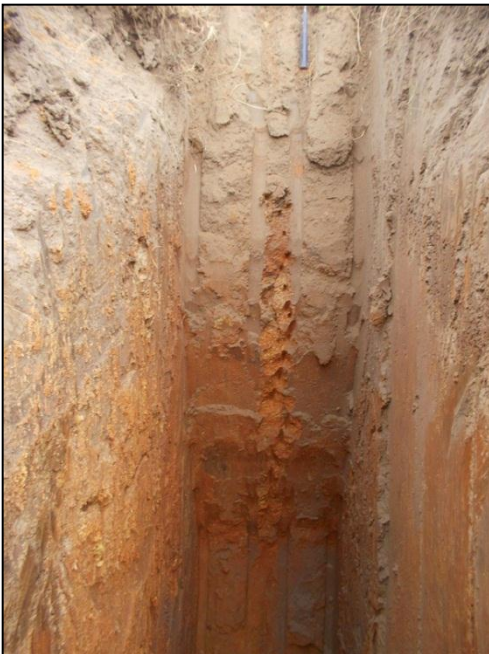
Note: Hole stopped TLB soft excavation.
