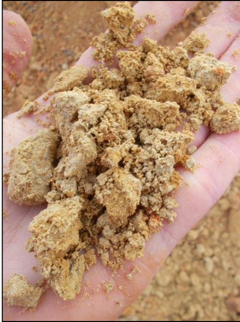
Note: Sandy silty material excavated.
