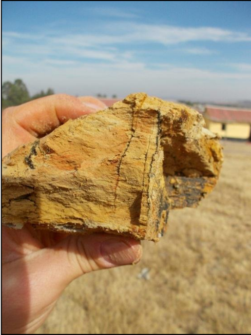
Note: Weathered shale fragment.
