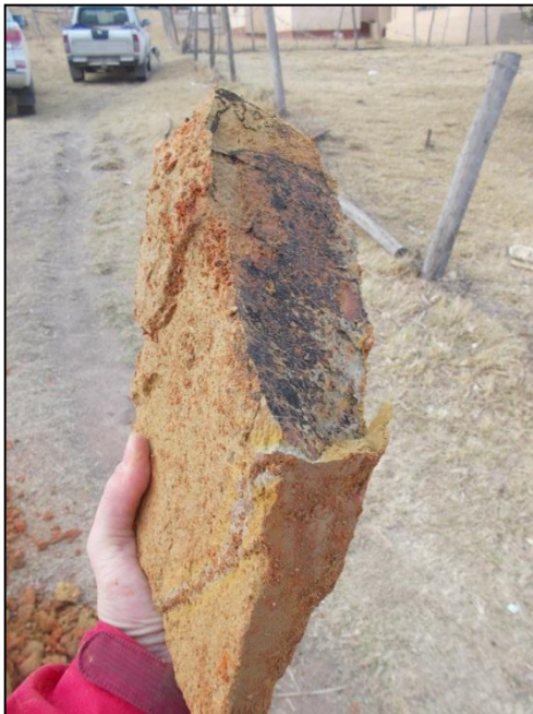
Note: Highly weathered shale fragment.
