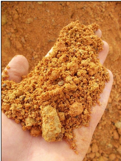
Note: Clayey silty material from excavated weathered shale.
