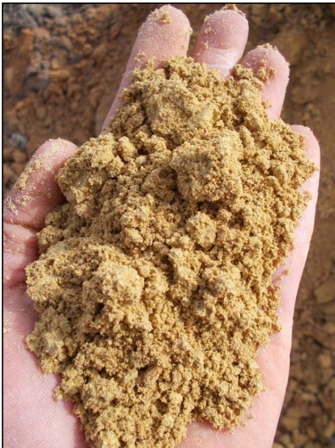
Note: Silty material of completely weathered shale.
