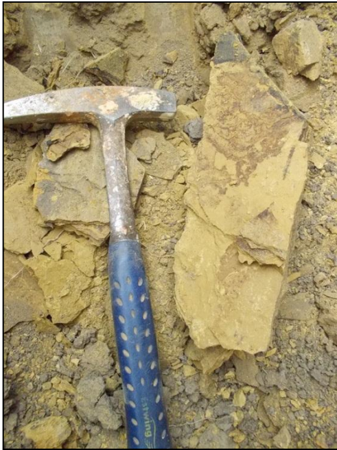
Note: Soft rock shale at base of test pit.
