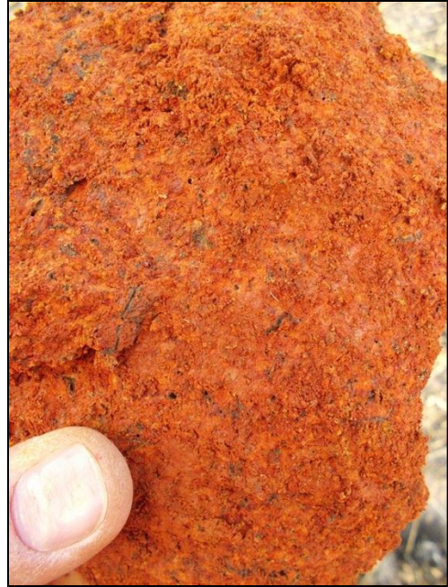
Note: Pinholed structure in profile.
