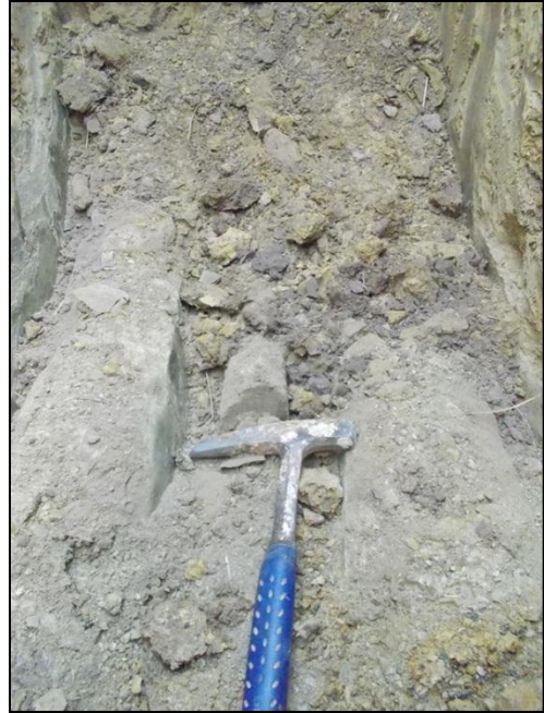
Note: Refusal of TLB on soft rock shale.
