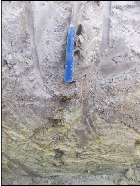
Note: Shallow refusal of TLB on soft rock shale.
