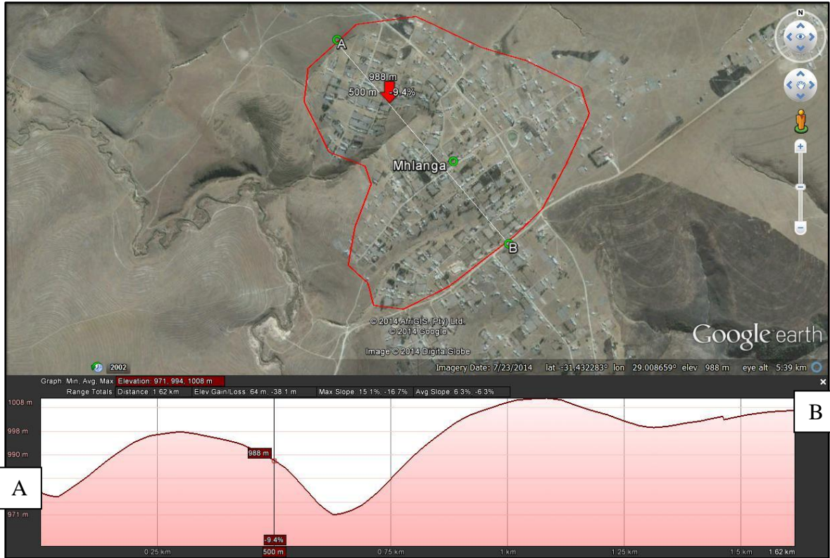
Figure R1: Elevation profile from north-west to south-east cross cutting the drainage feature in the valley.
