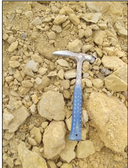
Note: Very soft rock shale fragments.
