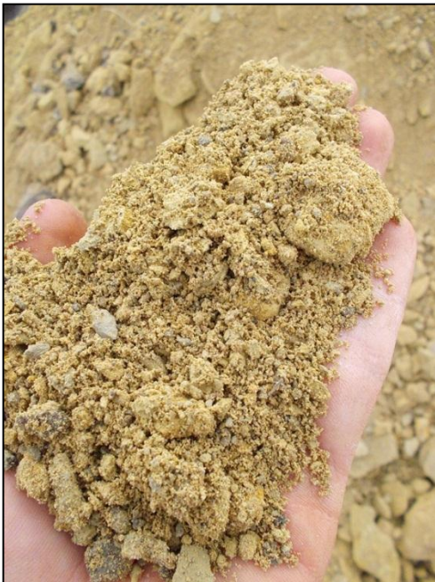
Note: Clayey silty material excavated.
