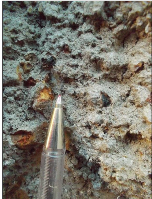
Note: Iron and manganese nodules in profile.
