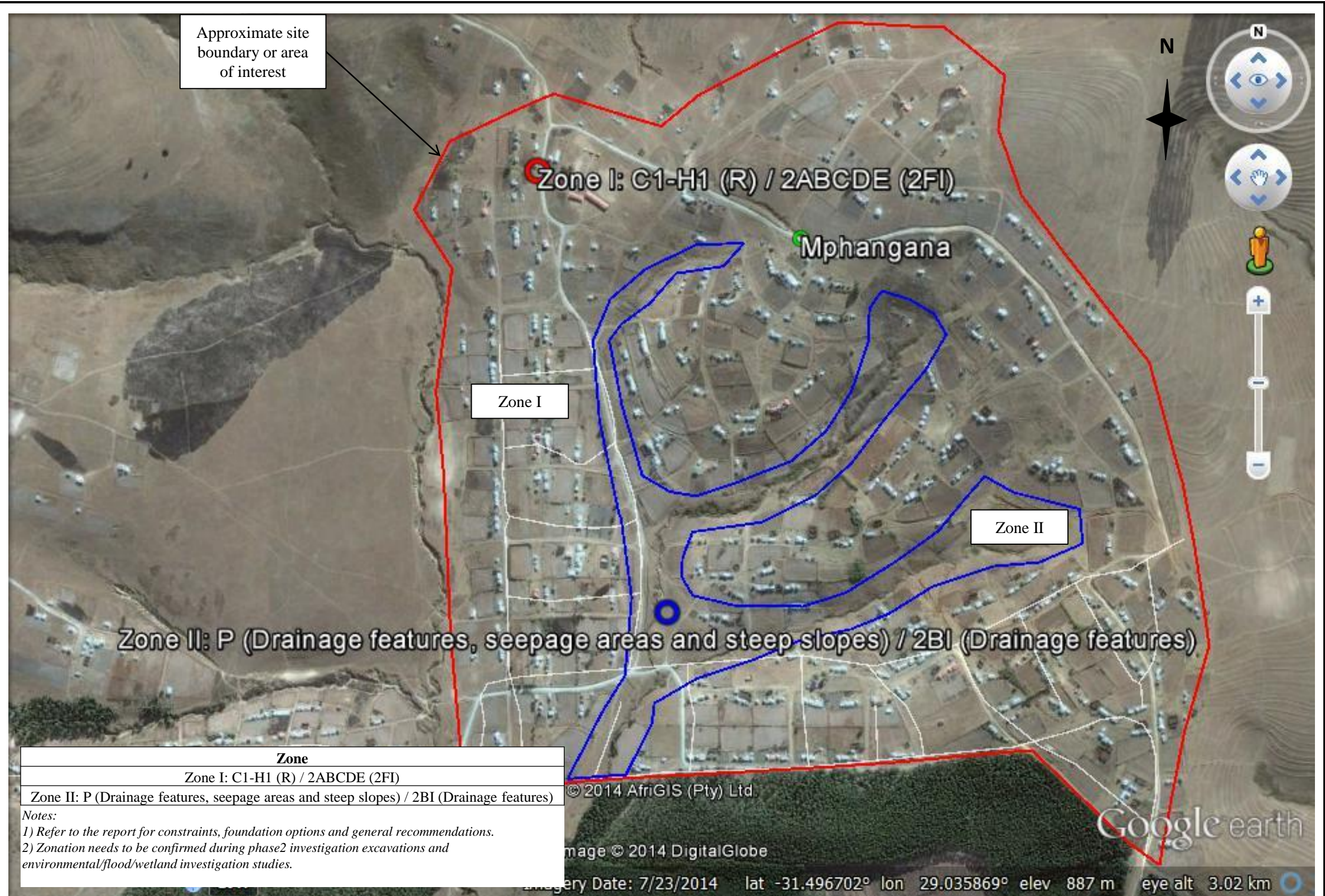
Figure 6: Geotechnical Zonation: Eastern Cape Housing (Mphangana)
