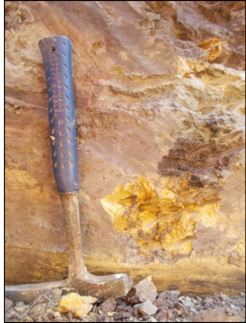
Note: Soft rock shale at base of test pit.
