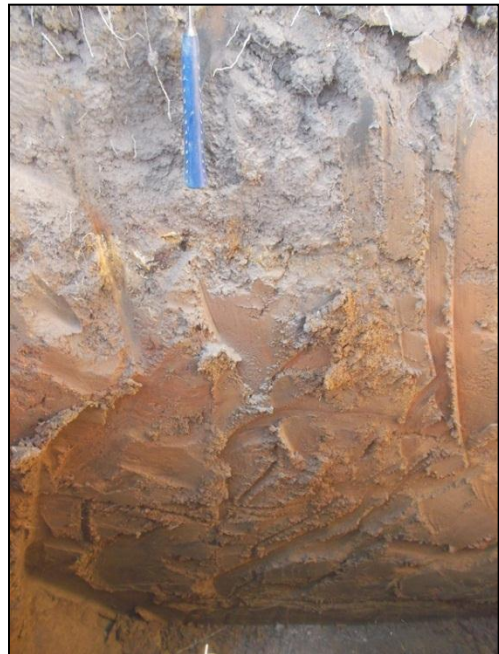
Note: Refusal of TLB on large boulder or bedrock.
