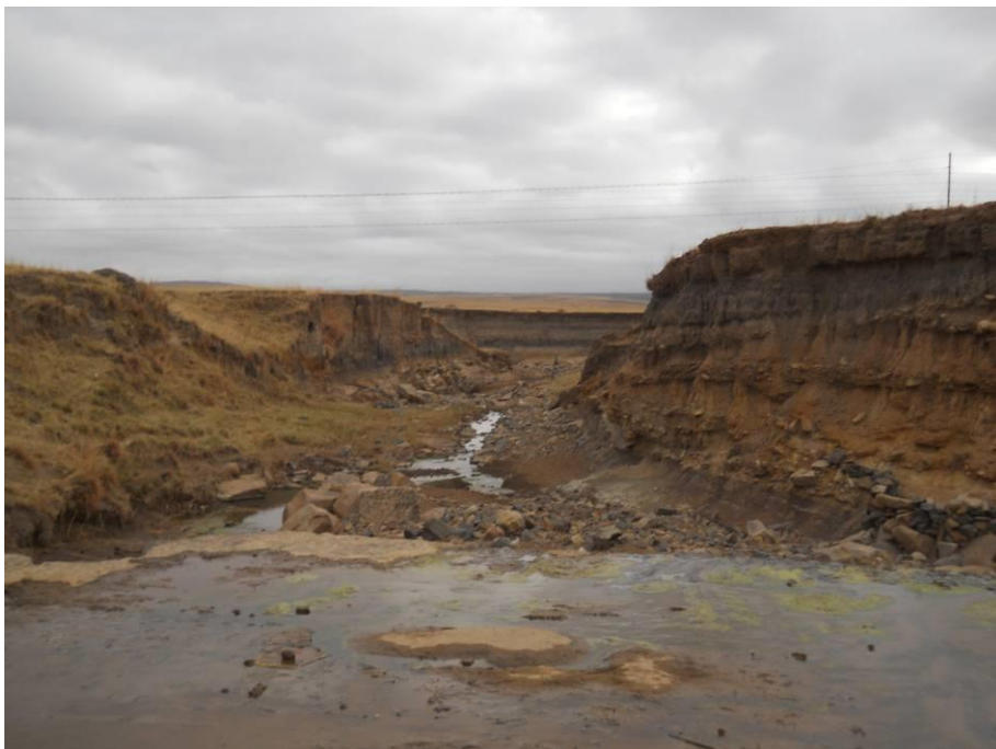
Figure 7.5 Thick scree and alluvium along the middle slopes, no outcrop of Elliot Formation mudstone (GPS 30 25 0.9S; 28 33 9.7E)
