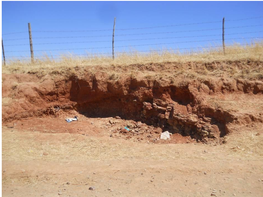
Figure 7.11 Typical deep soil cover on weathered Burgersdorp Formation mudstone, no fossils observed.
