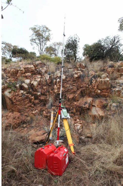
Figure 4. DGPS. A Leica Differential Geographic Positioning System set up over the WBMD1 datum.
