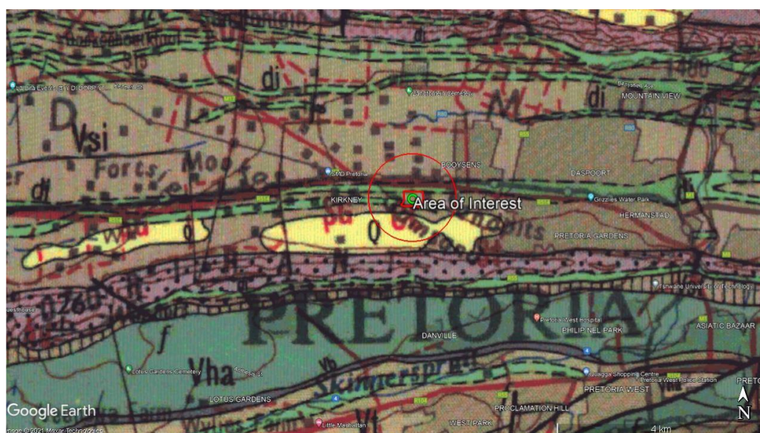
Figure 3: 1: 250 000 scale geological map (2528 Pretoria; 1:250 000 series) showing the position of the proposed shopping centre development (red quadrangle) on Portion 216 and Portion 36 of the Farm Zandfontein 317-JR, Tshwane Metropolitan Municipality, Gauteng Province. Di – diabase intrusion; Vdg – Daspoort Formation; Vsi – Silverton Formation; Q Quaternary alluvial deposits.
