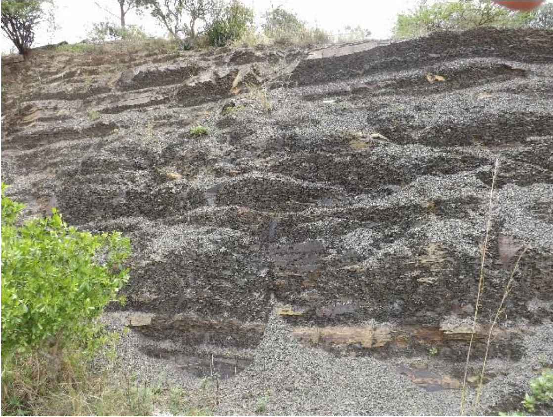
Figure 3: Example of the Volksrust Formation. This lithology is typically a blue shale and very weathered.
