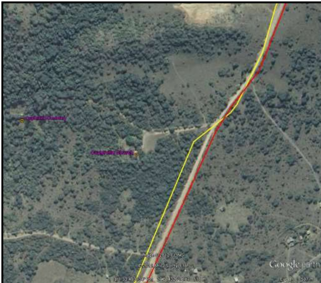
FIG. 33: PROPOSED RE-ALIGNED ROUTE (IN RED)
