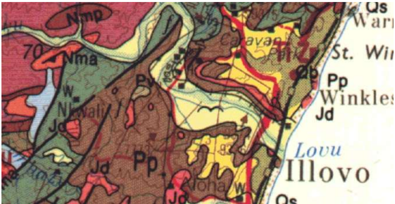
Figure 2: Approximate area of the Tranquility Memorial Park project. Extract from the 125 000 Geological Map: Port Shepstone 3030. According to this map the Pietermaritzburg Formation (Pp: Brown, Dwyka Group (C-Pd:Greenish) and probably the dolerite, sills or dykes, are present (Jd: Red).
