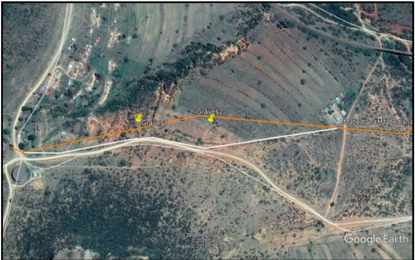
FIG. 15: OPTIONS 1 AND 2 FOR THE PIPELINE ROUTE 1
