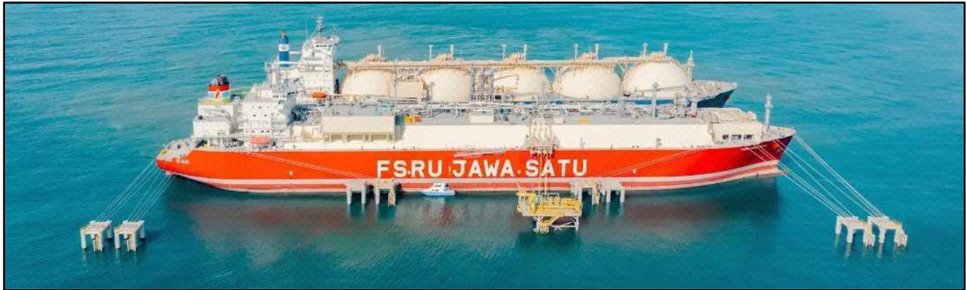
Figure 2-7: Example of FSRU and LNG carrier alongside secured with dolphin mooring system.
