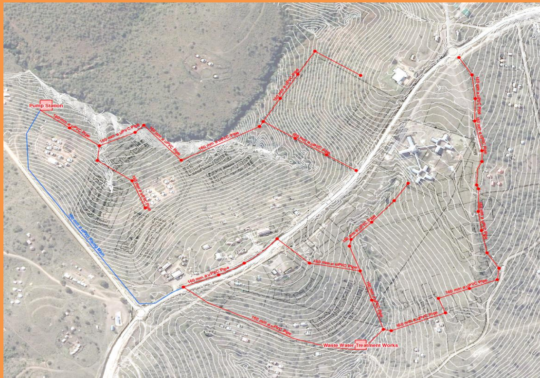
Figure 6: The sewer reticulation Alternative 2
