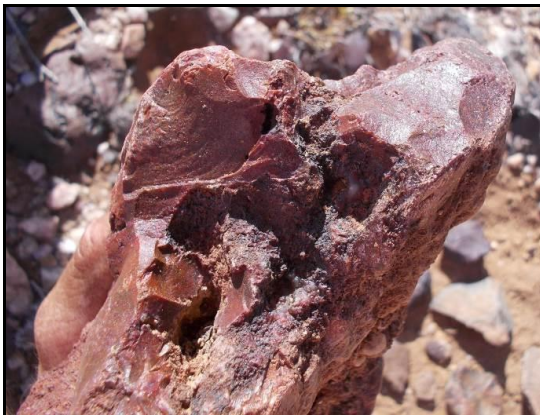
Figure 28 & 29: Two views of a core from the southwest side of G13. It shows flaking of the better quality parts of the rock. The material is either banded iron formation or silcrete.
