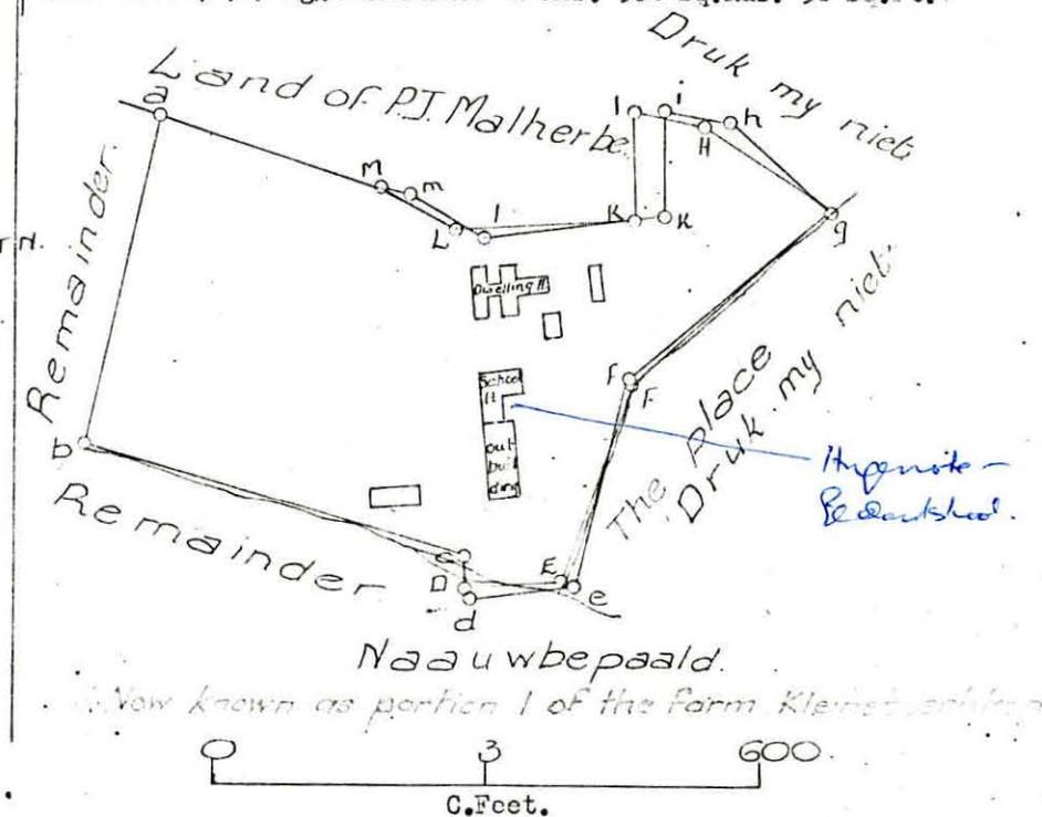
The above diagram a.b.c.D.d.e.f.g.h.i.K.J.m. represents 2 Morgen 487 Sq.Rds. 10 Sq.Ft. of Freehold situate at Daljosaphat F.C. Klein Drakenstein Division of the Paarl being part b of certain piece of land marked H transf'd together with another piece marked I. to S.J. du Toit, E.J. du Toit and others on the 10th January, 1899.
